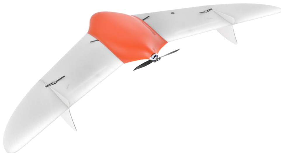
Picture 1 – The unmanned aerial survey system Geoscan 201.
